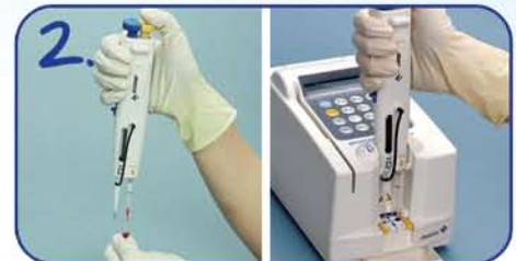
Draw the sample and reference solution with the twin-pipette. Set pipette and apply sample to E-plate
